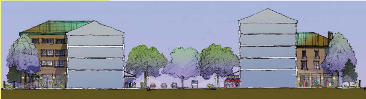
Figure 40: Mathis Avenue Section (indicating proposed 'main street' and courtyards at building rear)
